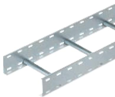
Cable ladder with 110 mm side height with welded C profile rungs which are open in an upwards direction. Rolled side rail for reinforcement and as edge protection. Fastening to the bracket takes place using clamps, type LKS 40. The slot dimension of the frame is 16.5 mm and the appropriate clamp clip is type 2056.
