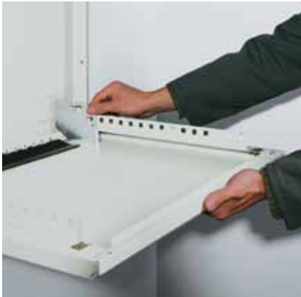
Slide the floor into the longitudinal slits provided and secure it with corner connectors, which are then fastened into place by screws
