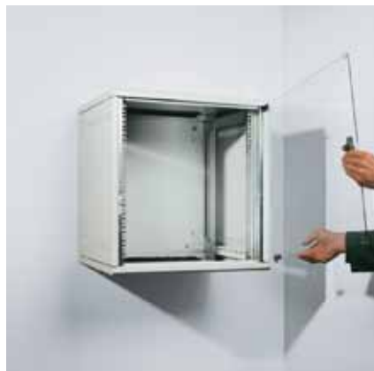
Mount the 482.6 mm (19") angles in the required position and slide the left and right hand side panels into place. Then, install the glass door by inserting the hinge pin into the top drill hole first, before allowing the bottom pin to slide into the lower hole. Secure the door at the top with the red securing ring
