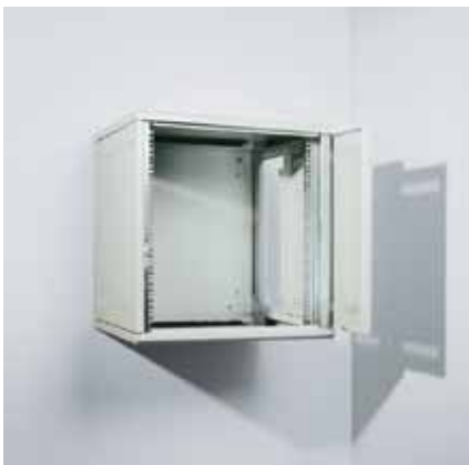
Mount the 482.6 mm (19") angles in the required position and slide the left and right hand side panels into place. Then, install the glass door by inserting the hinge pin into the top drill hole first, before allowing the bottom pin to slide into the lower hole. Secure the door at the top with the red securing ring
