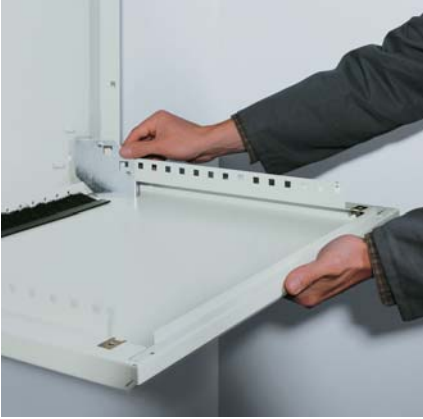
2 Slide the floor into the longitudinal slits provided and secure it with corner connectors, which are then fastened into place by screws
