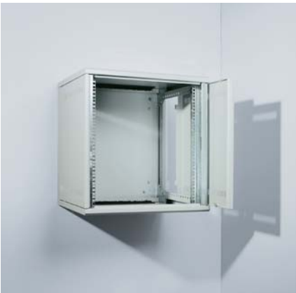
5 Mount the 482.6 mm (19") angles in the required position and slide the left and right hand side panels into place. Then, install the glass door by first inserting the hinge pin into the top drill hole, before allowing the bottom pin to slide into the lower hole. Secure the door at the top with the red securing ring
