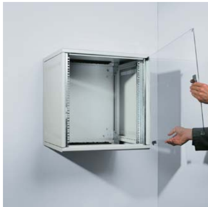
5 Mount the 482.6 mm (19") angles in the required position and slide the left and right hand side panels into place. Then, install the glass door by first inserting the hinge pin into the top drill hole, before allowing the bottom pin to slide into the lower hole. Secure the door at the top with the red securing ring
