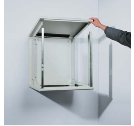
4 Place the roof on the top of the vertical mounting angles and bolt into place. Insert corner connectors and screw them tight
